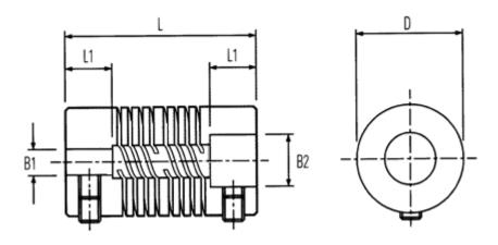
B1: Pre-drilled = 10.0B2: Pre-drilled = 16.00 D = 50.8 L = 95.3 L1 = 25.0 Max angular displacement = 0.90 = 28.00
